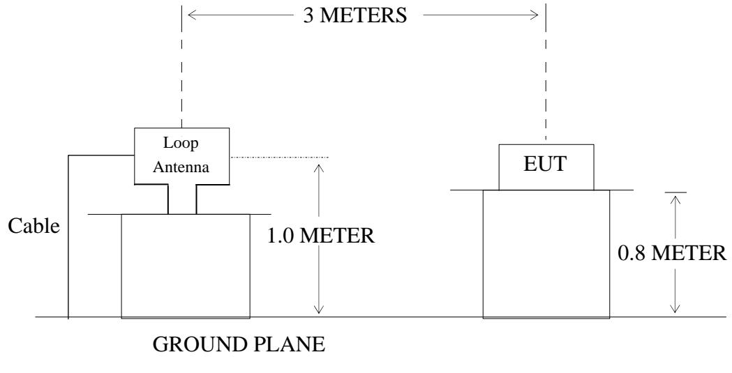
(EUT: Radio Control Transmitter)
