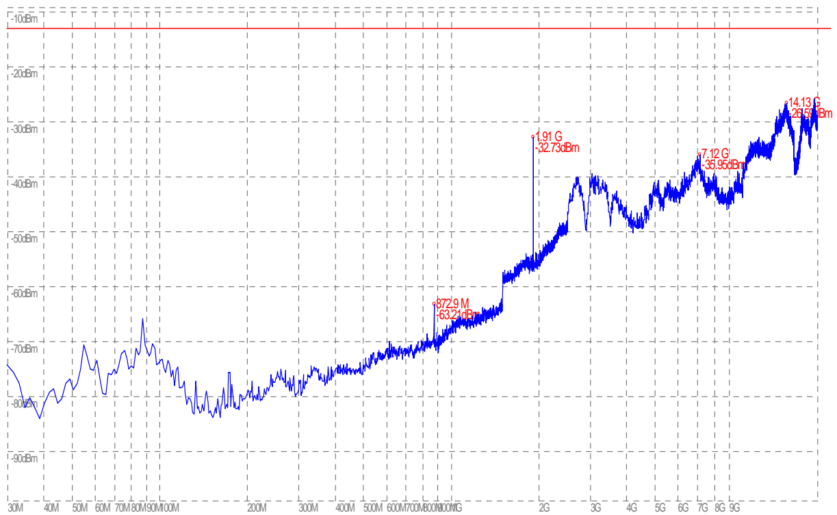
(Plot F.1: GSM 1900MHz Channel = 810, Test Antenna Horizontal)
