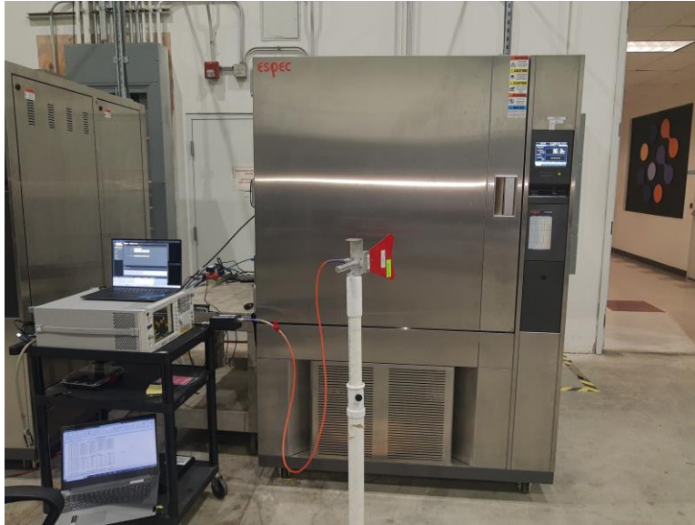
Photograph 1. Frequency Stability Setup
