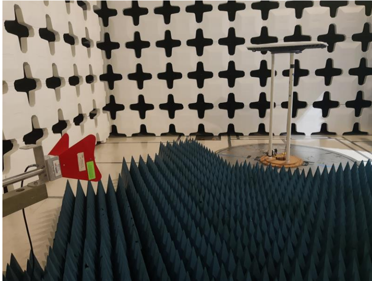
Photograph 3. RE Setup [1 GHz - 18 GHz]
