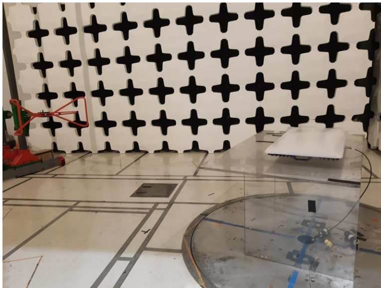
Photograph 2. RE Setup [0.03 GHz - 1 GHz]
