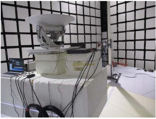
Radiated emissions measurements 18GHz to 26.5 GHz
