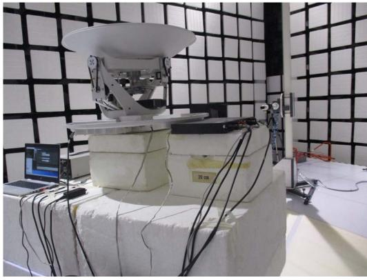
Radiated emissions measurements 26.5 GHz to 40 GHz
