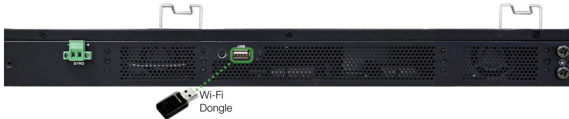
Figure 14: Back Panel Wi-Fi Dongle Connection
