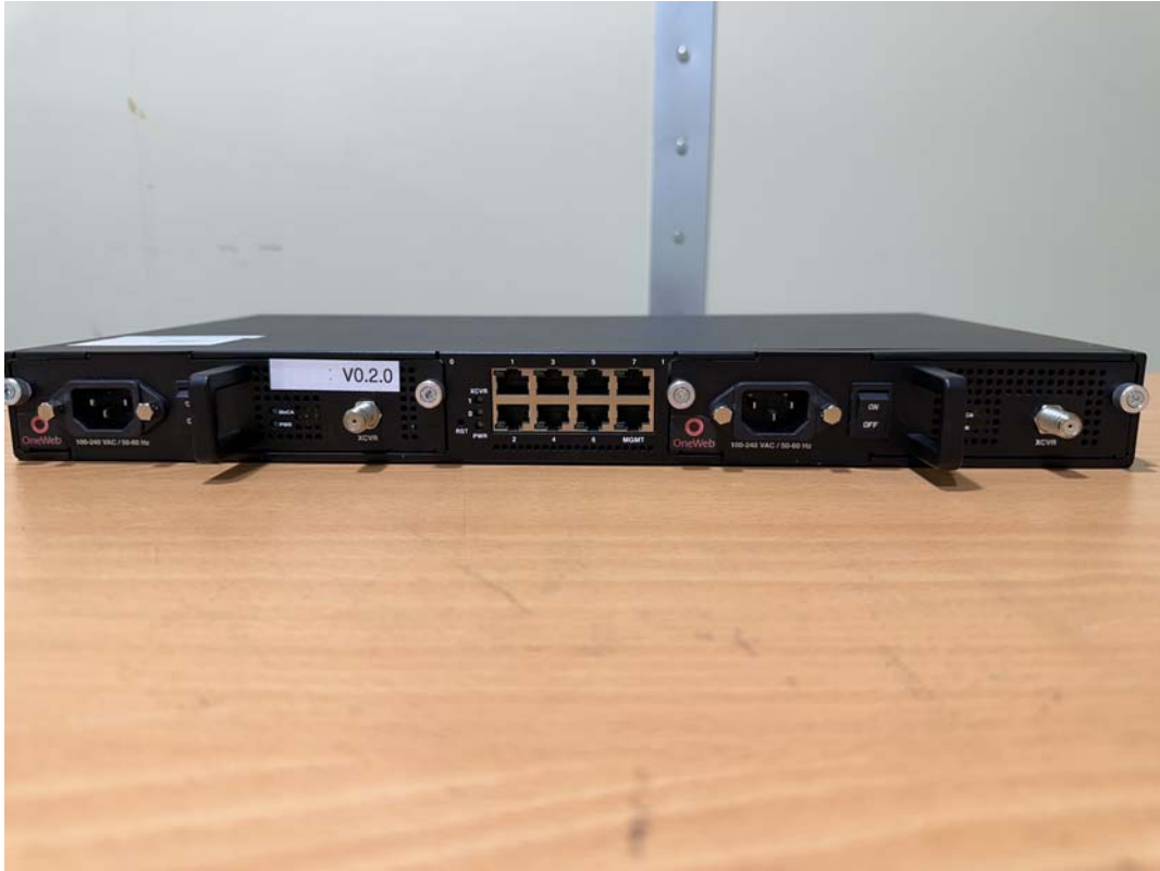
Customer Network Exchange I/O port
