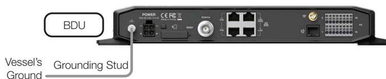
Figure 43: Grounding Stud Connection
