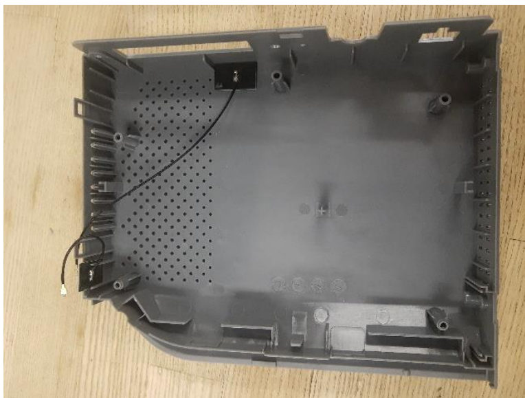
Figure 10: CNX-WiFi, Internal 5 GHz Antenna Position
