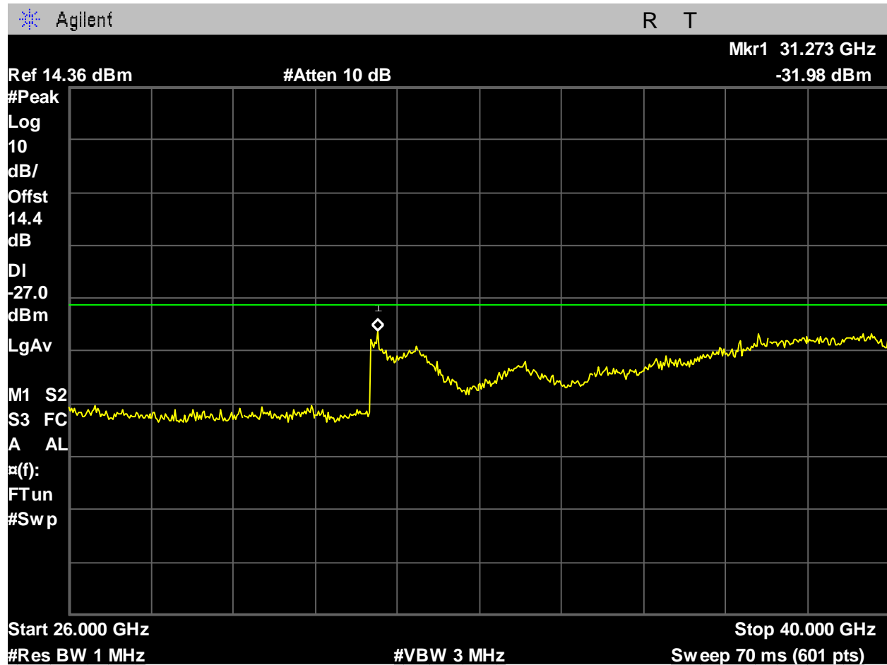
Figure 1252: U-NII-2A_5260MHz_low_mid Ch_52_20MHz BW_n-mode_-27dBm_26-40GHz_Port 1.
