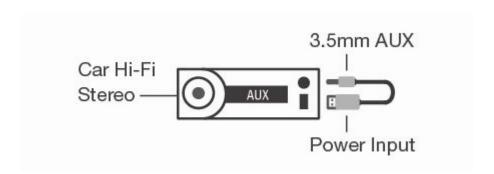
Car stereo system supporting only 3.5mm AUX jackPlug USB side of Uark into USB jack on USB car adapter (not included). Plug 3.5mm AUX side into AUX jack on car stereo. If too short, use the included extension cord.
