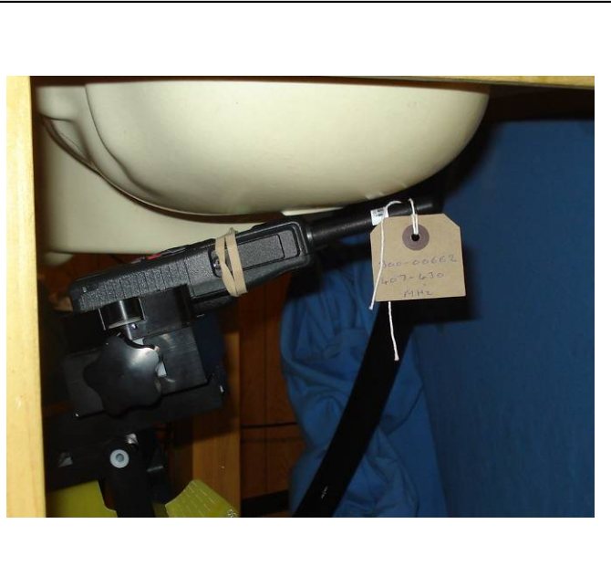
Held-to-Ear Test Setup – STP9240, -00662 Antenna, Left ear tilt position
