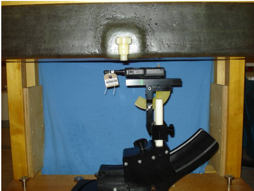
Face-Held Test Setup – STP9240, -00662 Antenna, -00635 Battery
