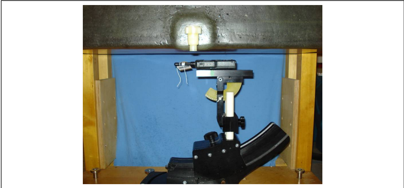
Face-Held Test Setup – STP9240, -00662 Antenna, -00634 Battery
