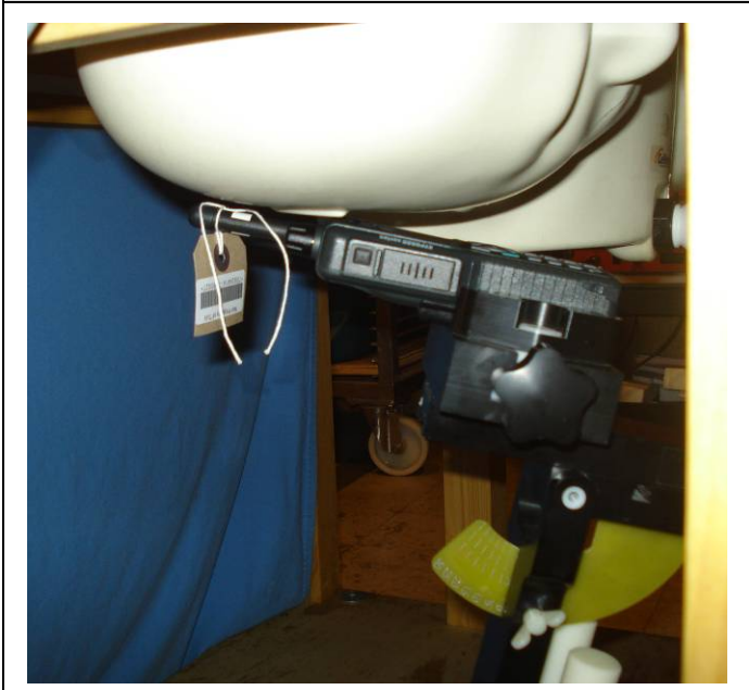
Held-to-Ear Test Setup – STP9040, -00663 Antenna, Right ear tilt position
