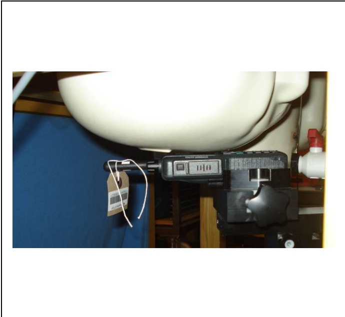
Held-to-Ear Test Setup – STP9040, -00663 Antenna, Right ear touch position
