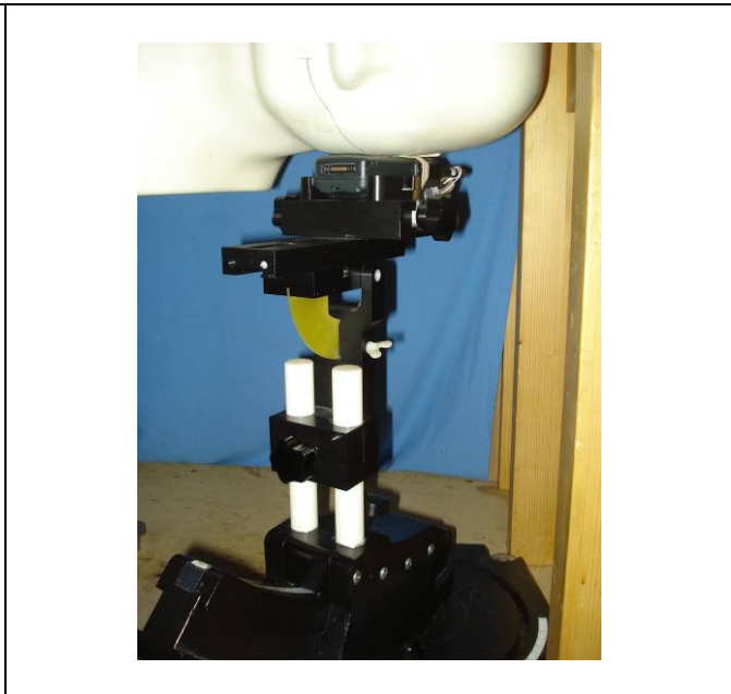
Held-to-Ear Test Setup – STP9240, -00662 Antenna, Left ear touch position
