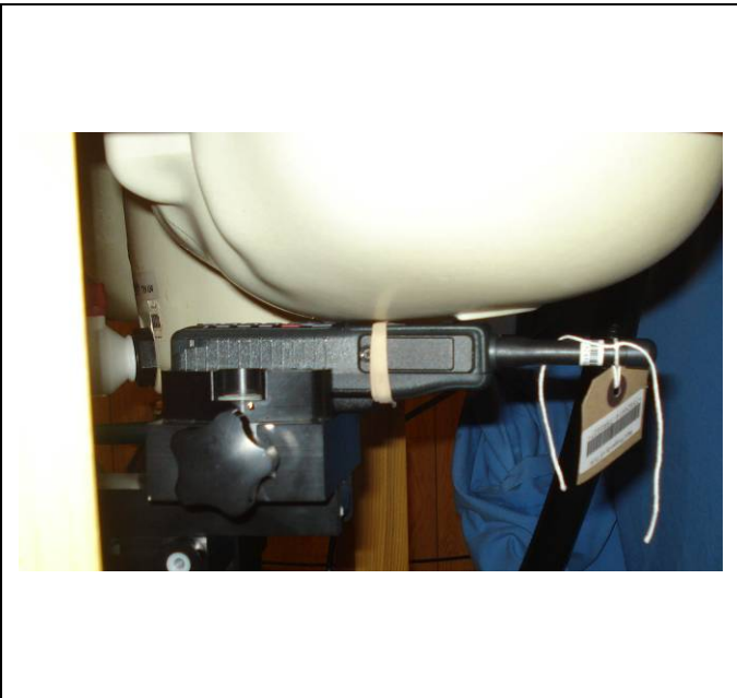
Held-to-Ear Test Setup STP9040, -00663 Antenna, Left ear touch position
