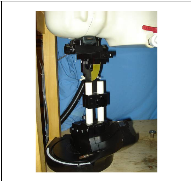
Held-to-Ear Test Setup – STP9240, -00662 Antenna, Right ear touch position
