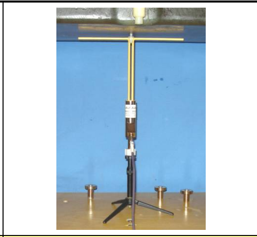
SPEAG 450 MHz Validation Dipole Setup
