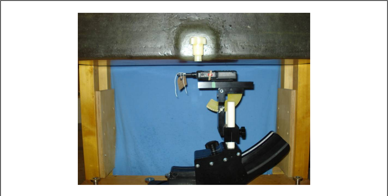
Face-Held Test Setup – STP9040, -00663 Antenna, -00635 Battery
