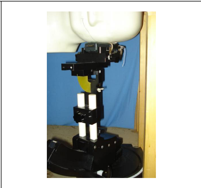
Held-to-Ear Test Setup STP9040, -00663 Antenna, Left ear touch position
