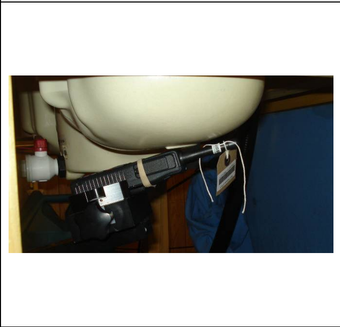
Held-to-Ear Test Setup – STP9040, -00663 Antenna, Left ear tilt position
