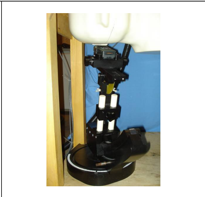
Held-to-Ear Test Setup – STP9240, -00662 Antenna, Right ear tilt position
