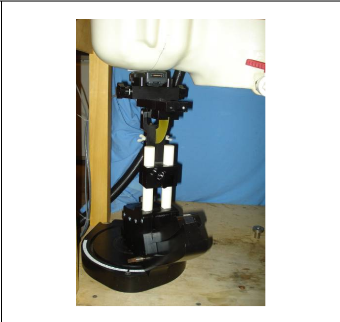
Held-to-Ear Test Setup – STP9040, -00663 Antenna, Right ear touch position
