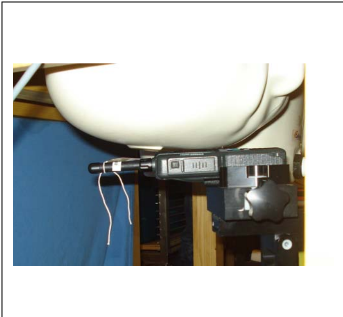
Held-to-Ear Test Setup – STP9240, -00662 Antenna, Right ear touch position
