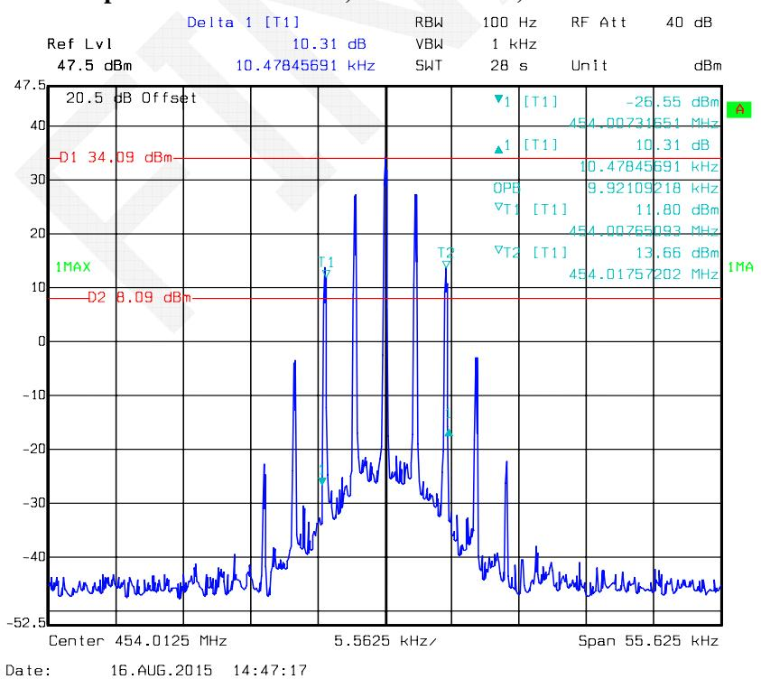
**Occupied Bandwidth –4FSK, 454.0125 MHz, High Power Level**
