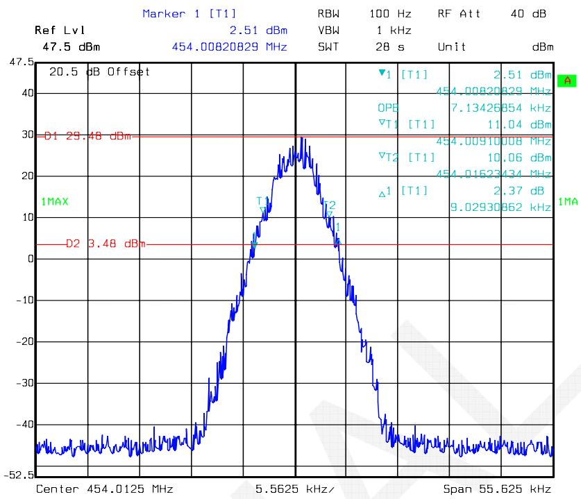
**Occupied Bandwidth –4FSK, 454.0125 MHz, Low Power Level**
