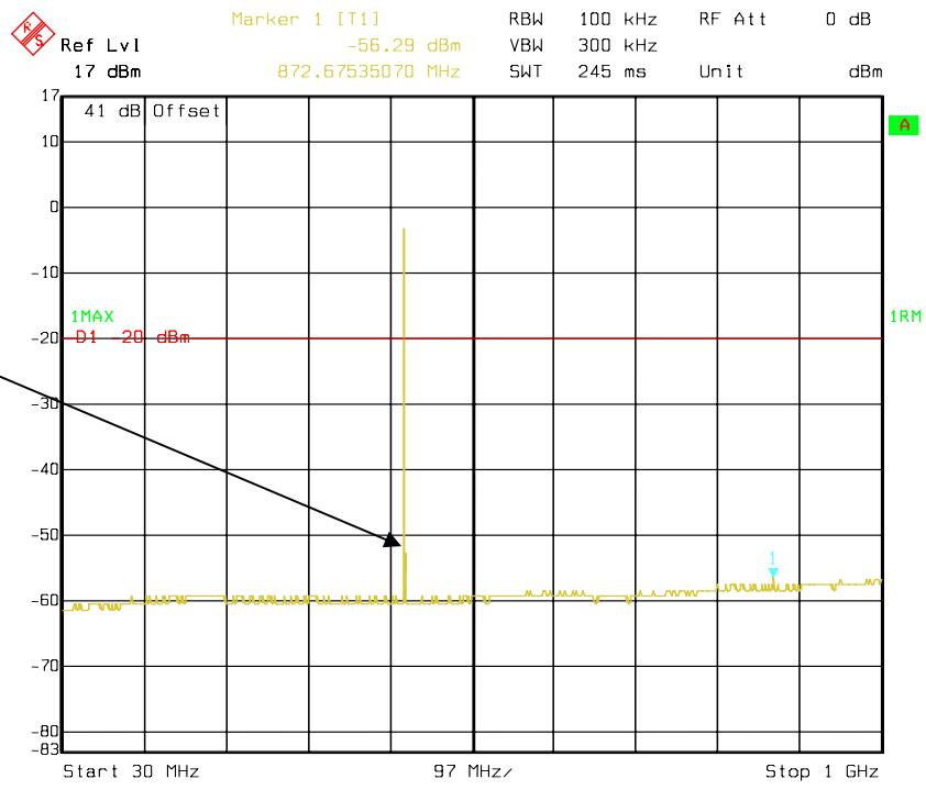
Fundamental test with Band Reject Filter
