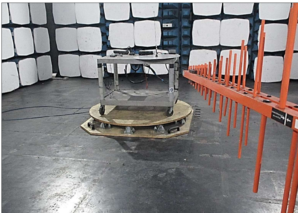
Figure 12 - Test Setup - 30 MHz to 1 GHz
