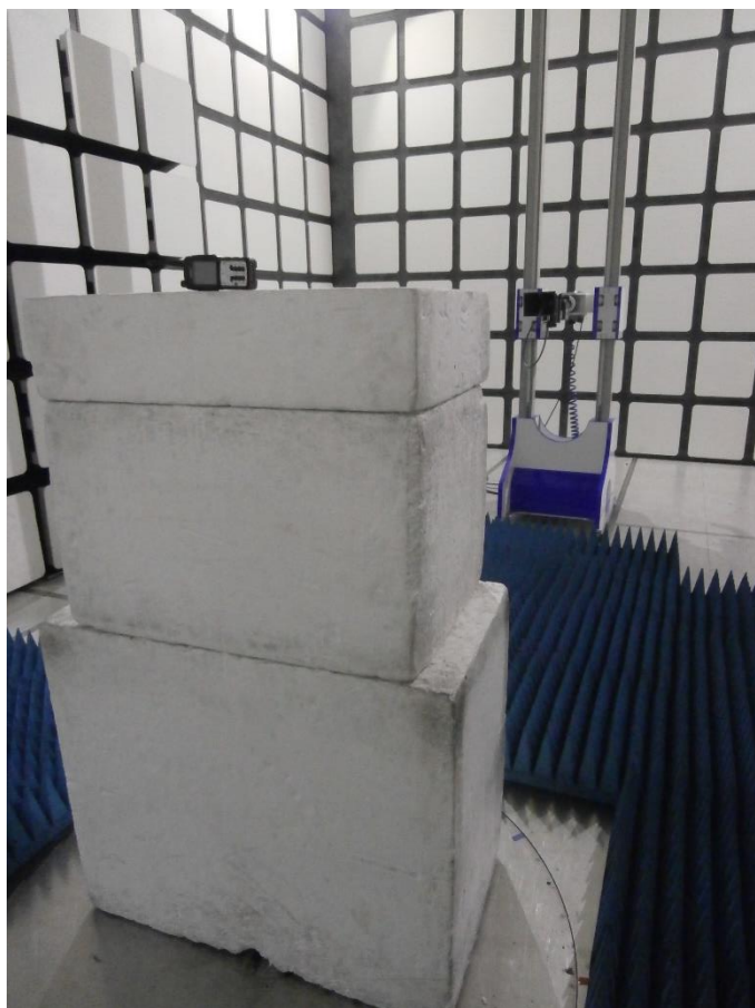
Figure 98 – Radiated Emission Setup, EUT Orientation Y
