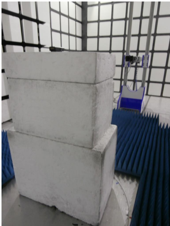
Figure 97 – Radiated Emission Setup, EUT Orientation X
