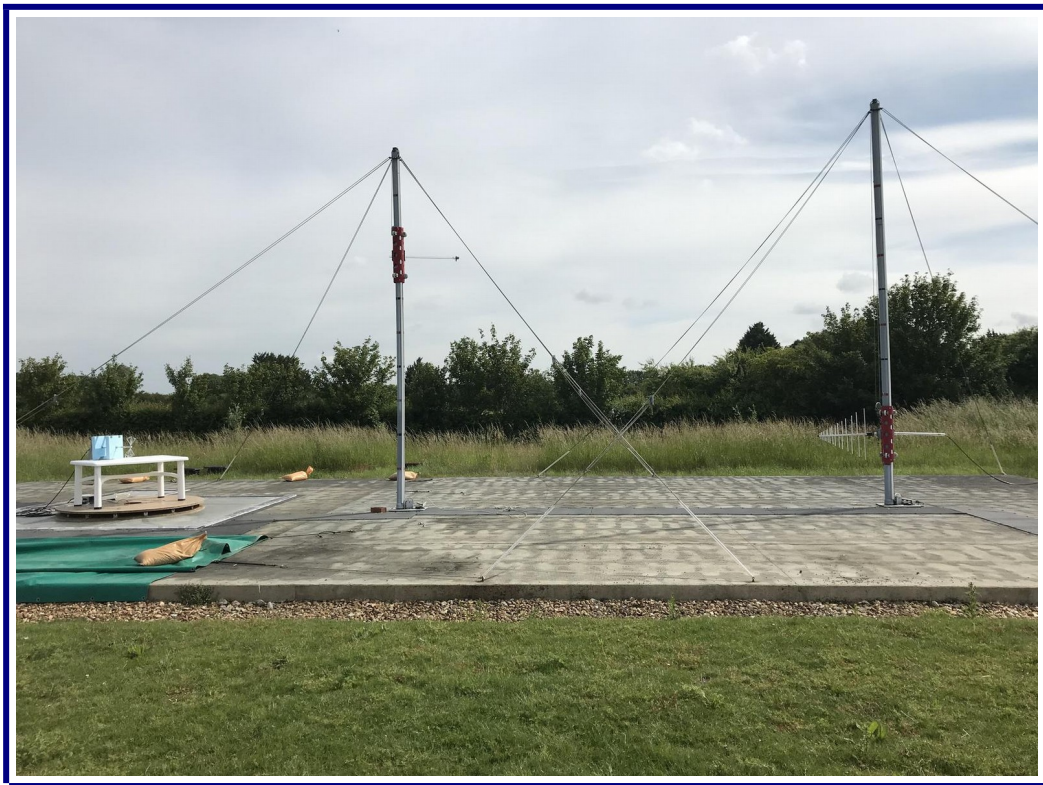
Photo 1: Substitution Measurement - 10m OATS
