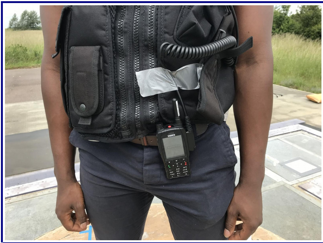
Photo 7: Belt worn RSM cable parallel
