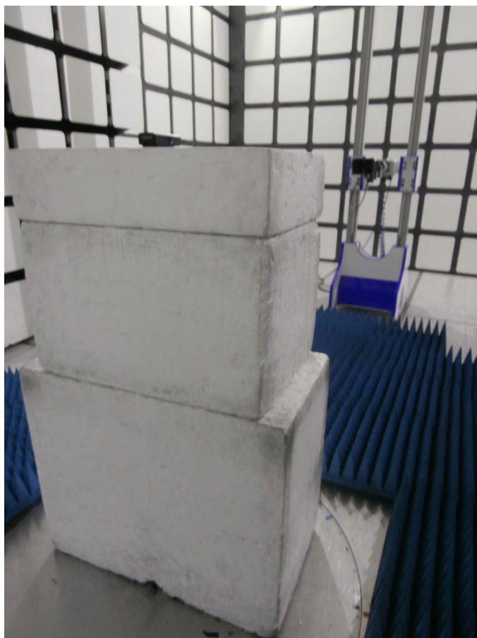
Figure 97 – Radiated Emission Setup, EUT Orientation X
