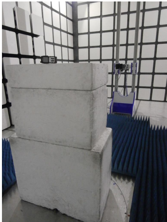
Figure 98 – Radiated Emission Setup, EUT Orientation Y
