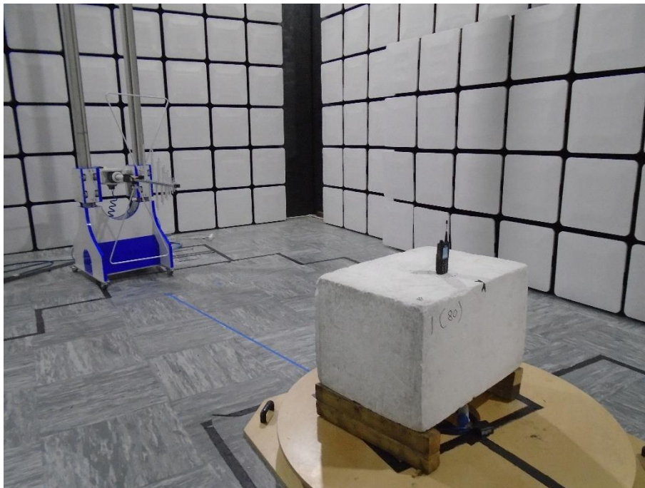
Figure 106 – Test Setup – 30 MHz to 1 GHz Z Orientation
