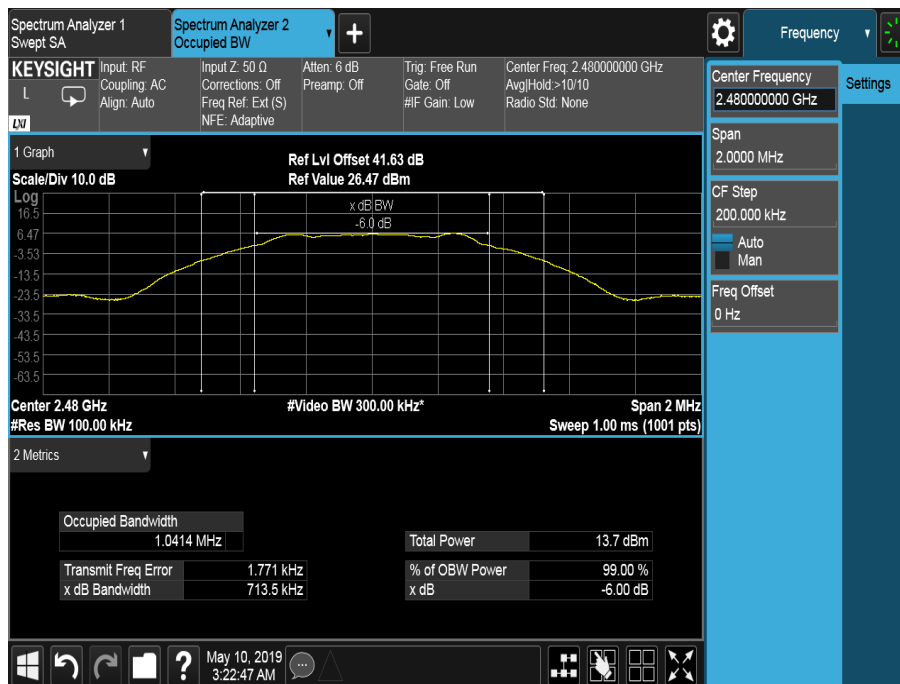
Figure 11- 2480 MHz – 6 dB Bandwidth & 99% Occupied Bandwidth
