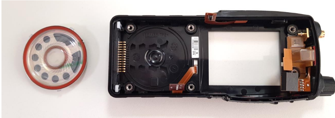
Figure 13. XX6SC2028 Front Cover with Speaker Removed
