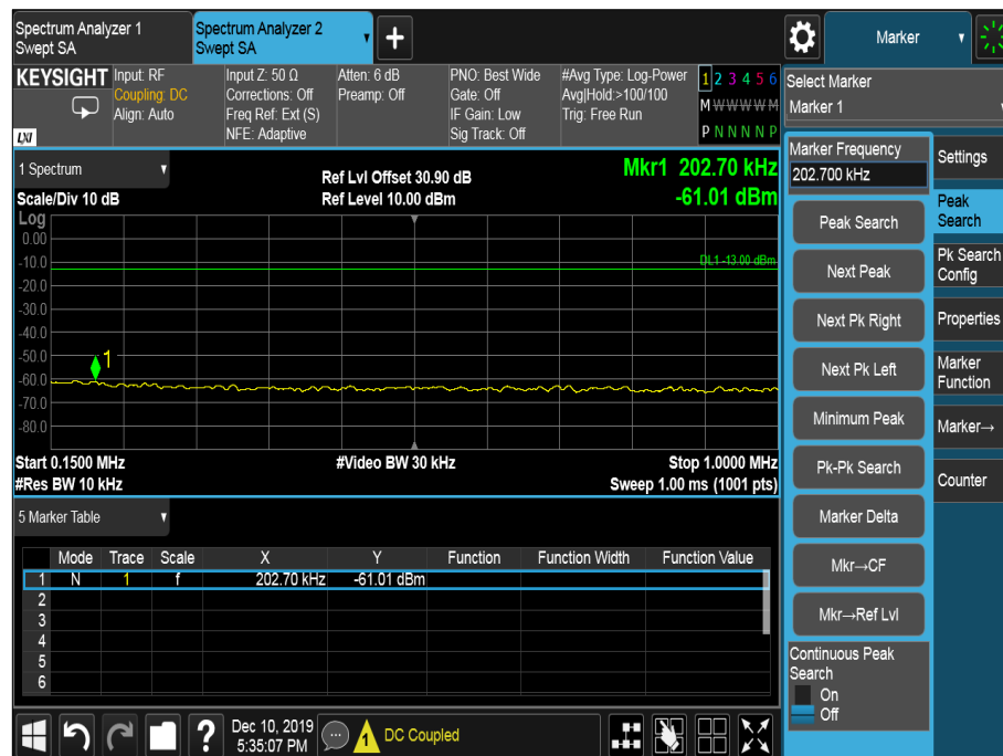
Figure 14 - 815.000 MHz, 150 kHz to 1 MHz
