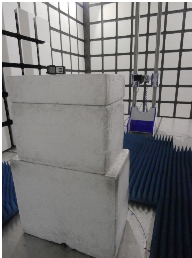
Figure 98 – Radiated Emission Setup, EUT Orientation Y
