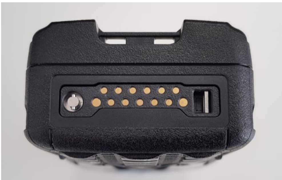
Figure 5. XX6SC2028 Underside with Battery Removed
