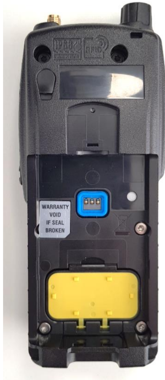
Figure 3. XX6SC2028 Rear with Battery and Antenna Removed
