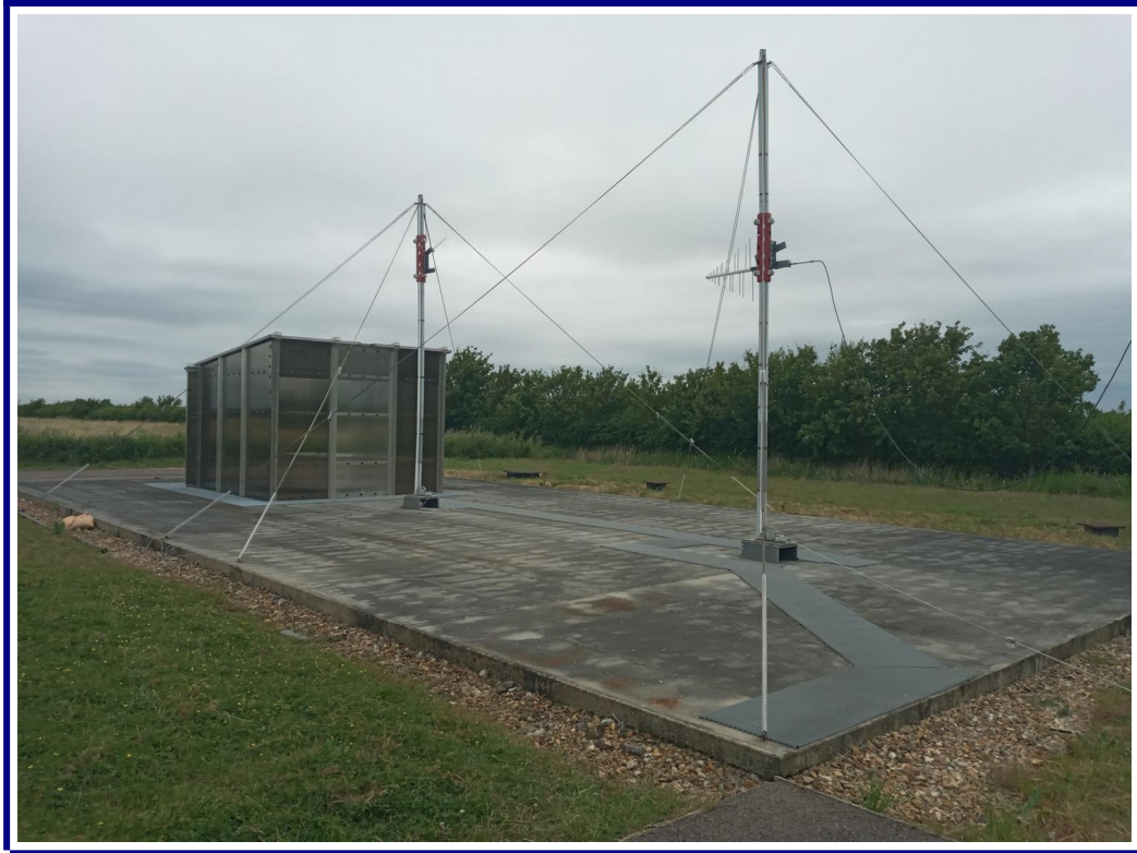
Photo 1: Radiated Emissions : Polar plot measurement setup
