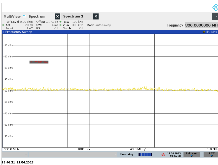
Figure 32 - 418.050 MHz, 600 MHz to 1 GHz Mask Y
