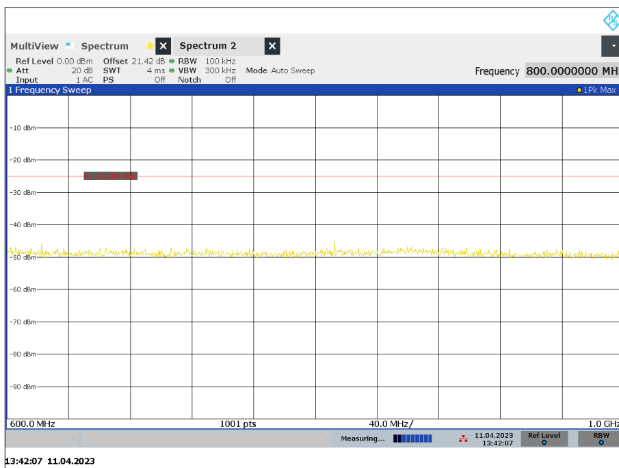
Figure 31 - 406.125 MHz, 600 MHz to 1 GHz Mask Y
