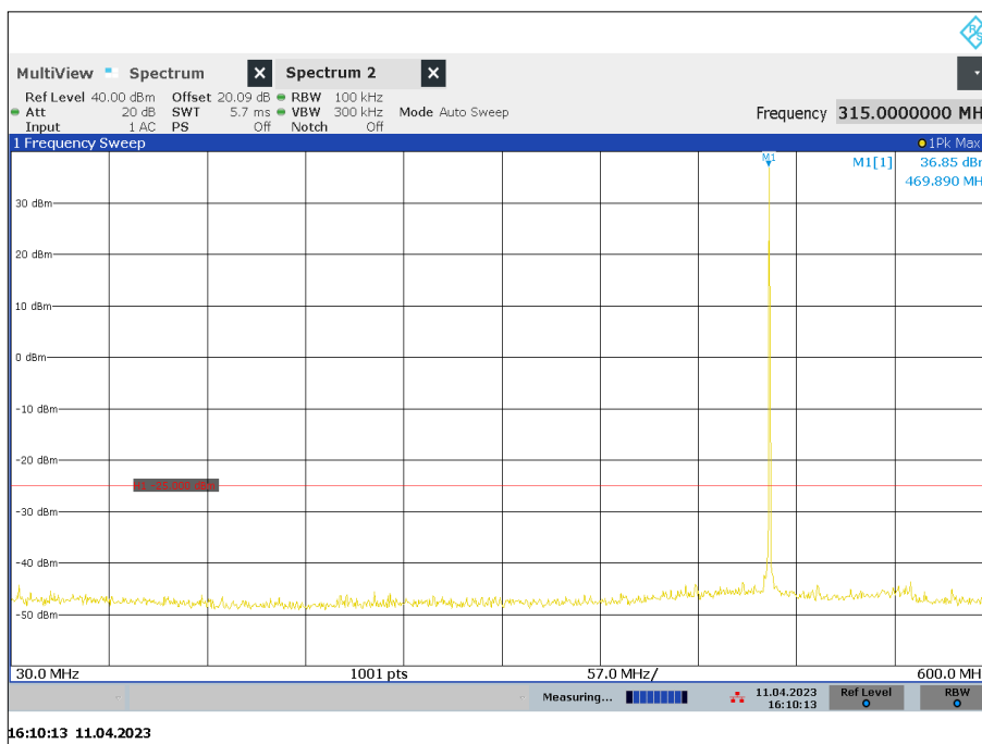
Figure 51 - 469.975 MHz - 30 MHz to 600 MHz Mask Y
