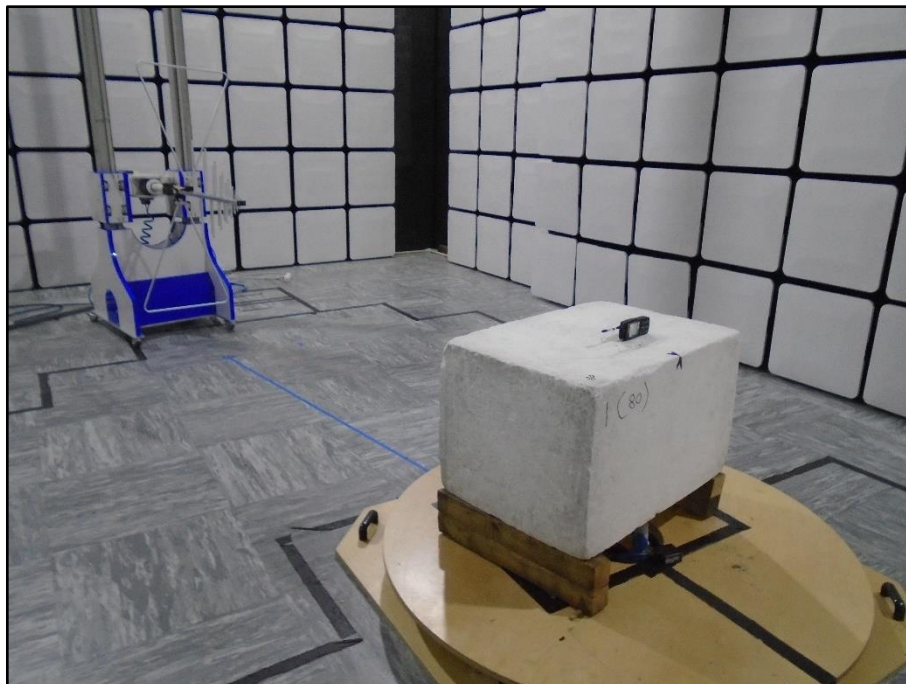
Figure 110 – Test Setup, 30 MHz to 1 GHz X Orientation
