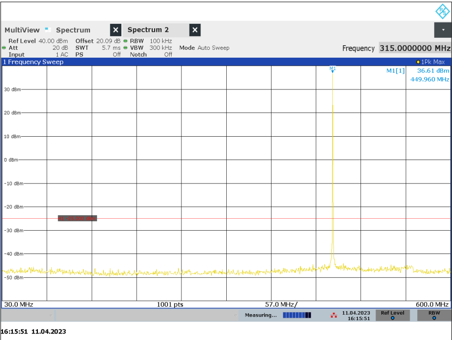
Figure 49 - 450.025 MHz, 30 MHz to 600 MHz Mask Y
