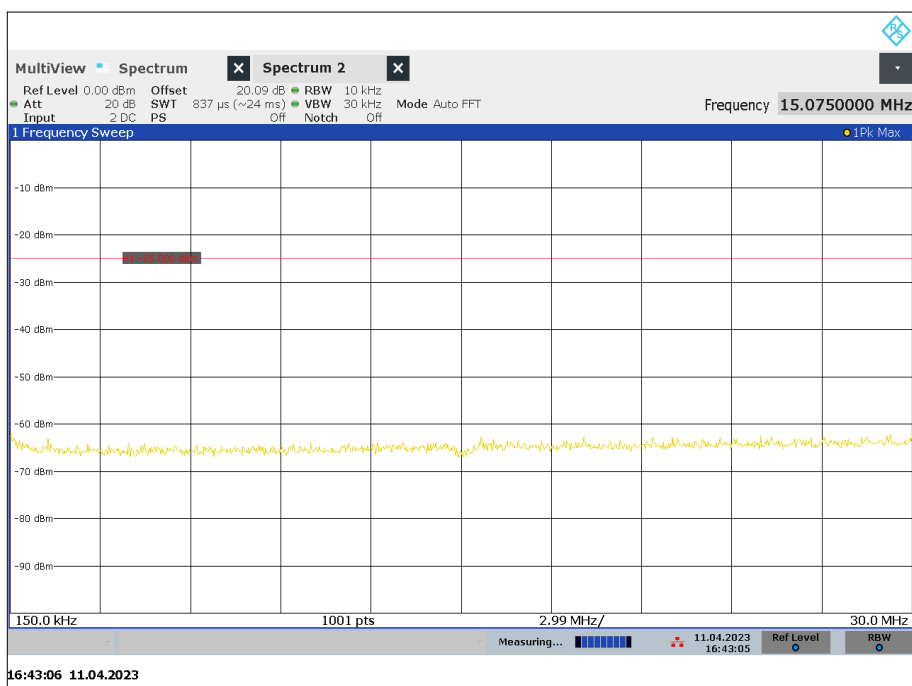
Figure 46 - 450.025 MHz, 150 kHz to 30 MHz Mask Y
