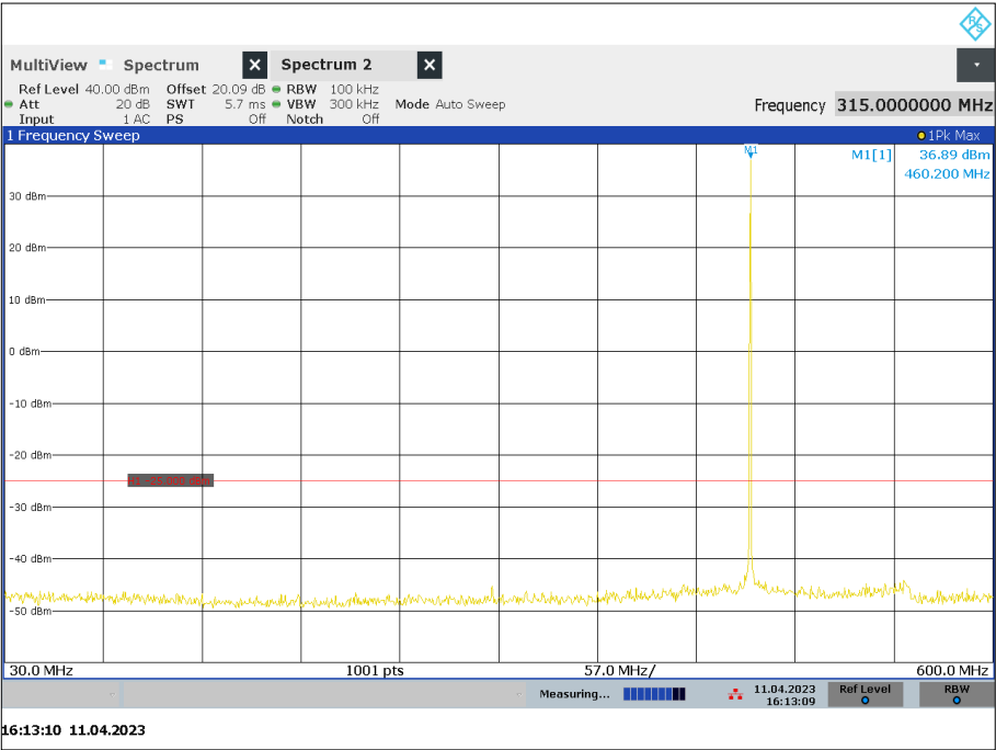
Figure 50 - 460.025 MHz, 30 MHz to 600 MHz Mask Y
