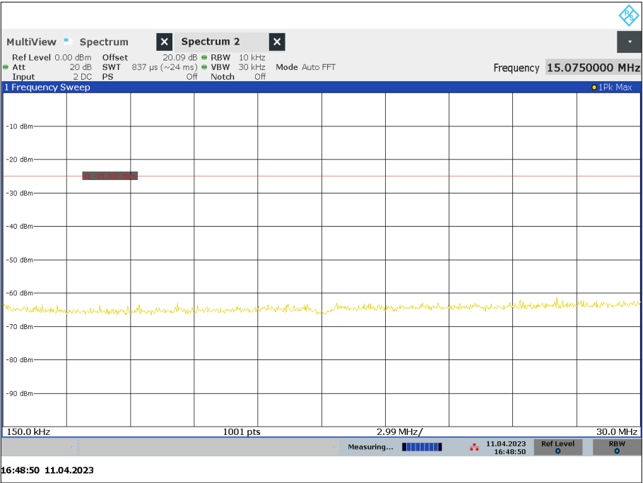
Figure 48 - 469.975 MHz - 150 kHz to 30 MHz Mask Y
