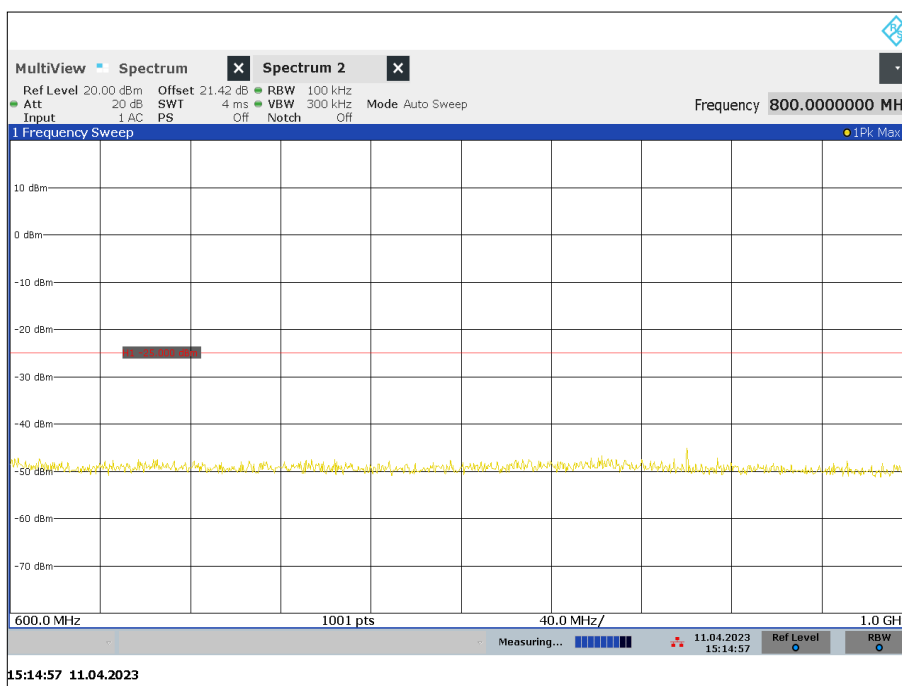
Figure 52 - 450.025 MHz, 600 MHz to 1 GHz Mask Y
