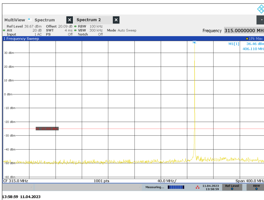
Figure 28 - 406.125 MHz, 30 MHz to 600 MHz Mask Y
