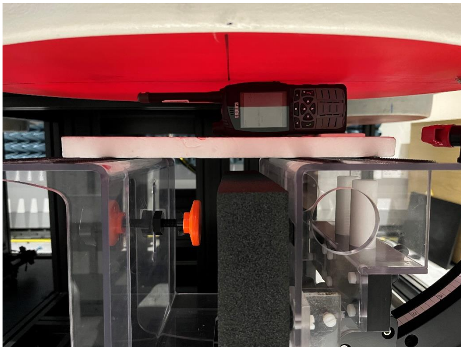
Figure C.8: DUT left right surface touching the body 0mm gap configuration.
