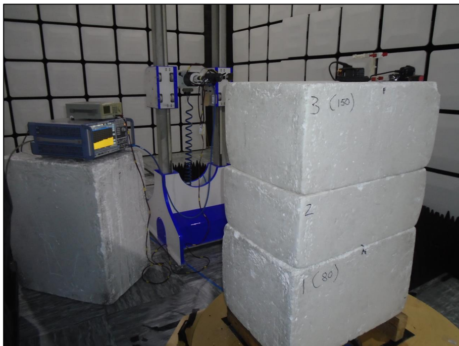
Figure 25 - Test Setup - 18 GHz to 25 GHz
