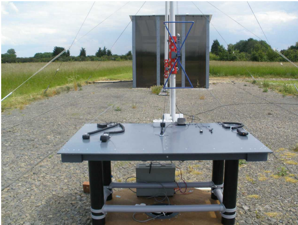
Photograph 2 Configuration 1: Radiated Emissions - Front
