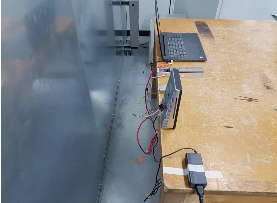
**- Radiated Emission Test****1) 125 kHz**
