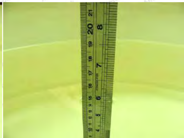
Photo of Liquid Height for Body SAR
