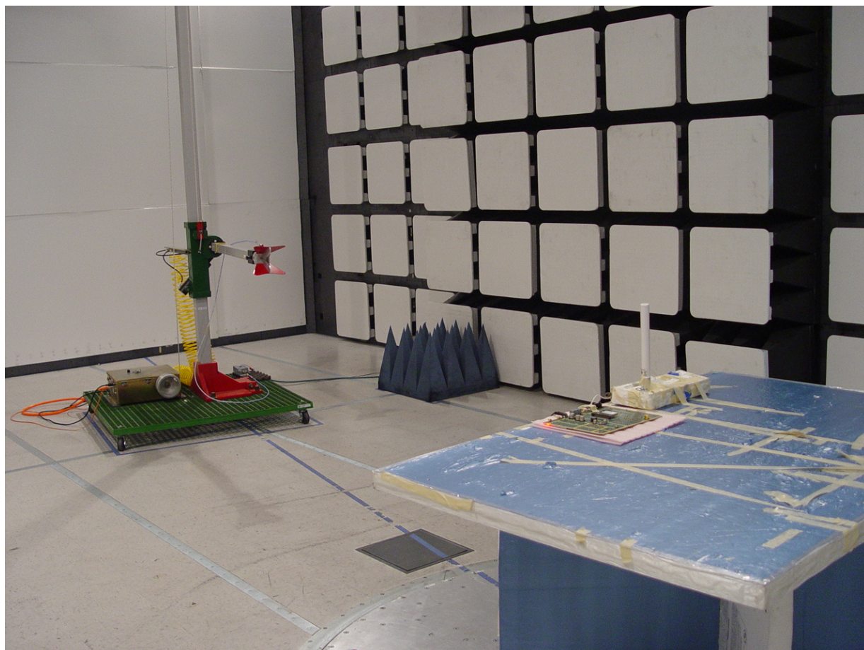
WiFi Module WLM54AG with omni directional antenna AIR-ANT2506 (gain 5.2 dBi)
