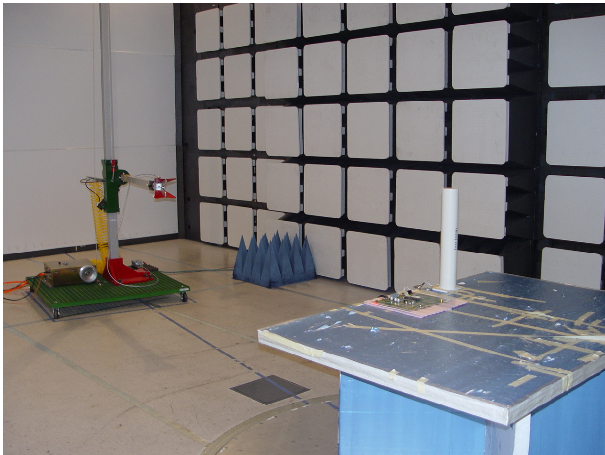
WiFi Module WLM54AG with yagi directional antenna AIR-ANT1949 (gain 13.5 dBi)
