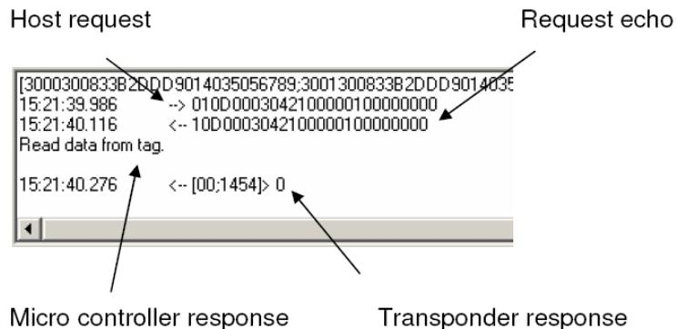
The relevant information returned by the Reader (transponder response, register content) is always in brackets to distinguish it from other data in host-to-reader data exchange.
