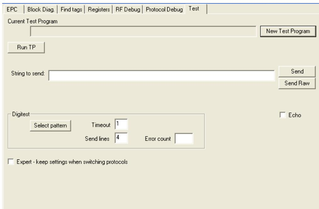
All Host to Reader commands that are described in the enclosed Interface description can be manually send in the Test tab using a string and the Send button. you simply has to fill the 'Command + parameters' field as shown. All other fields in the protocol are automatically generated by the program when **Send** button is pressed:
