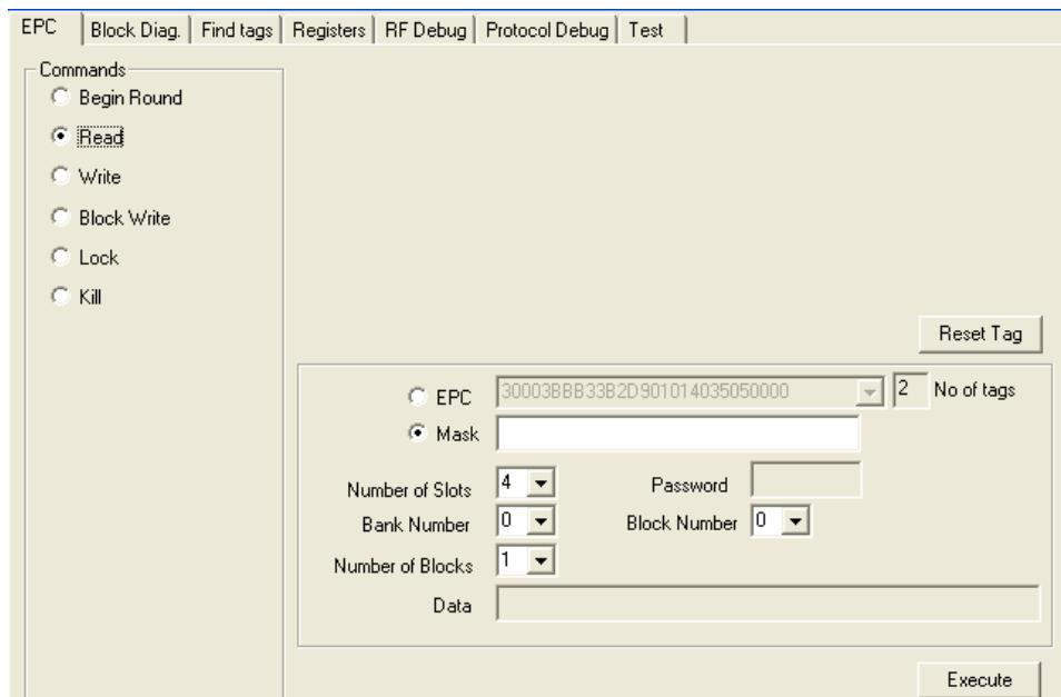
When this tab is activated only Inventory Round operation is enabled. You have to click Execute to run this operation and inventory the transponders before you can Execute other operations. When operations other then Inventory Round are selected modification of appropriate text entry and selection controls is enabled.
