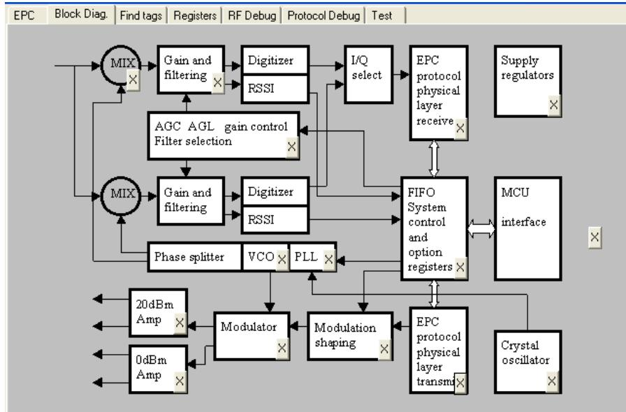
A block diagram of the circuit is presented to give a convenient possibility to change registers and modify properties of circuit blocks by clicking the **X** button in the lower right corner of some blocks. A new dialog box is opened where you can modify values of registers by entering new values in the text entry controls or selecting appropriate values from selection controls.
