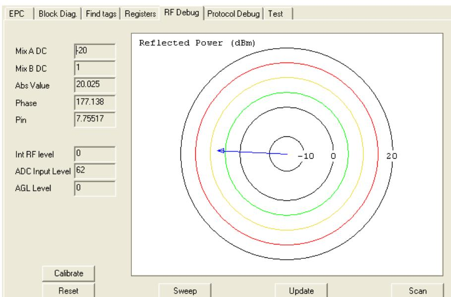
Update soft key is used update the readout on selected frequency. Scan soft key is used for continuously update. Sweep key is used to show results in a frequency domain using a wide frequency sweep. It is also possible to store the response shape by pressing calibrate key and in next sweep observe only the difference between actual reflectivity and the stored previous one.
