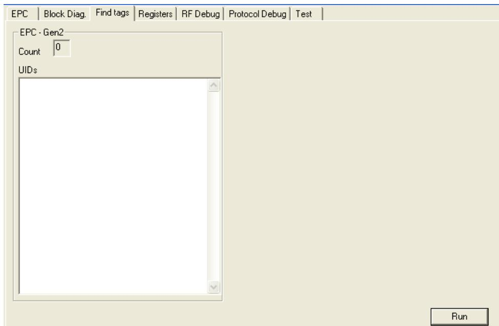
By changing into this tab, the active Reader is trying to identify all tags or labels in the RF field. The EPC numbers of the tags will be shown. This operation can be stopped and restarted with the **Stop / Run** button. No Reader to PC communication is echoed to the log window but it is still written to the log file (rfid-reader.log).
