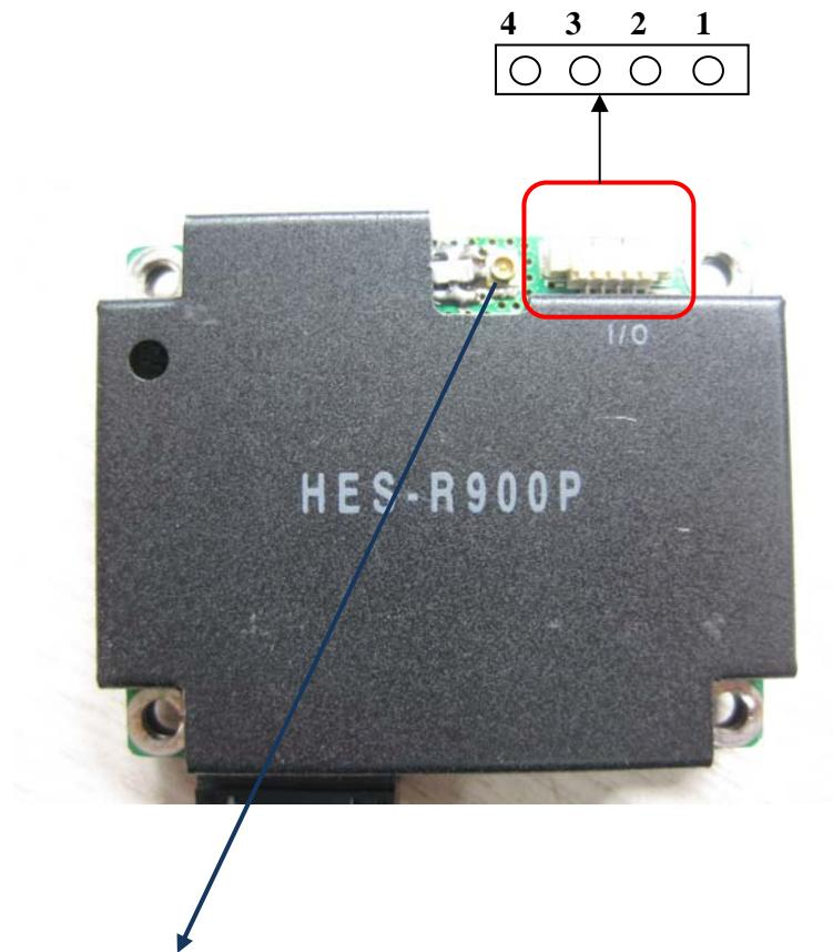
**Ant port :** connect rf cable to reader module and ANT
