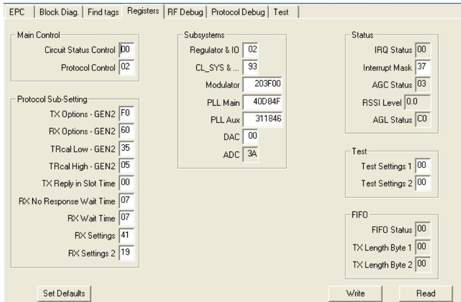
The content of the registers in AS3990 can be read and written in the **Registers** tab. Do not alter the register content unless you are familiar with the functions described in the AS3990 specifications. If you change the content by mistake, press the **Set Defaults** button. The register values are updated automatically every time the user enters the Registers tab or when the Special functions on the Main Window are changed.
