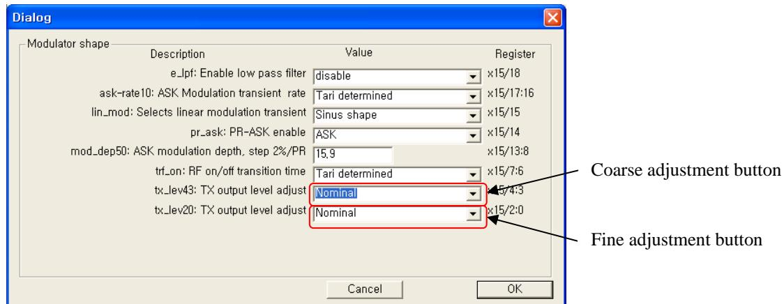
Be able to modified RF output Power of RFID board where Dialog window when click the Modulation shaping button.
