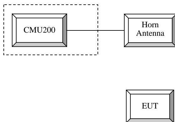
**Block Diagram of Test Setup**
