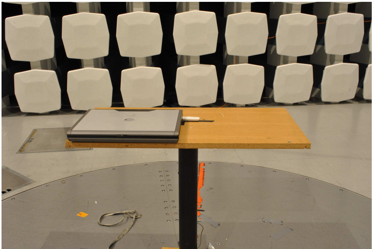
Set-up for Radiated spurious emissions 30 – 1000 MHz
