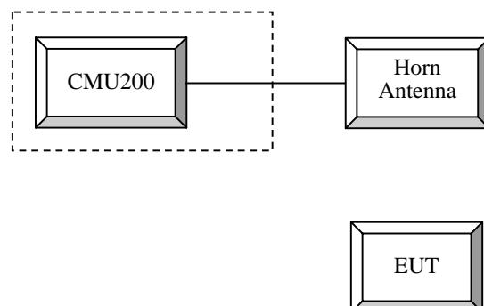
**Block Diagram of Test Setup**
