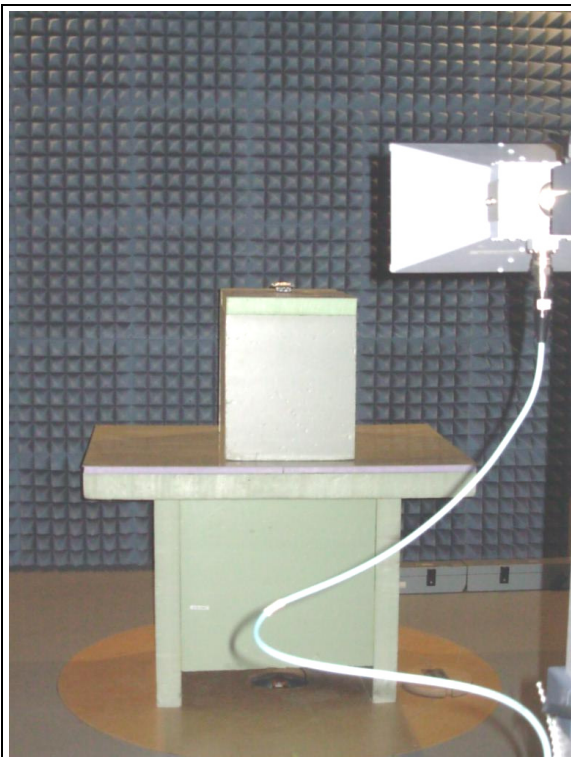
Figure 10: Measurement set-up for radiated measurement > 1 GHz acc. following sections of the report 1112-11-EE-11-PB001: 4.5.3; 4.5.4 and 4.6.2
