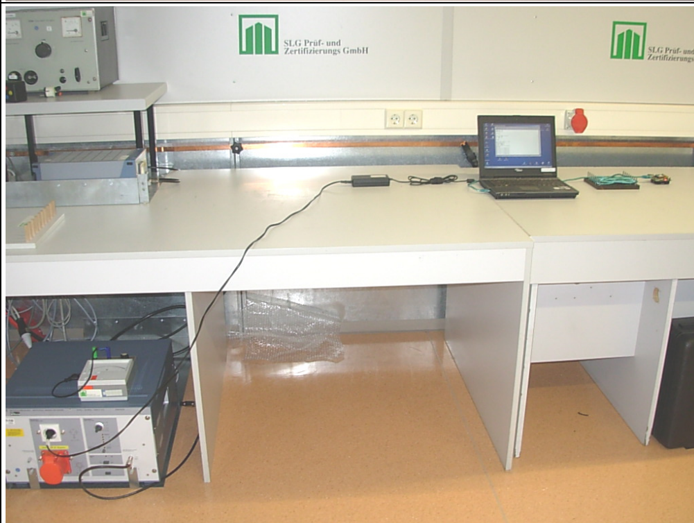
Figure 11: Measurement set-up for conducted measurement of disturbance voltage acc. following section of the report 1112-11-EE-11-PB001: 4.7 and 4.8
