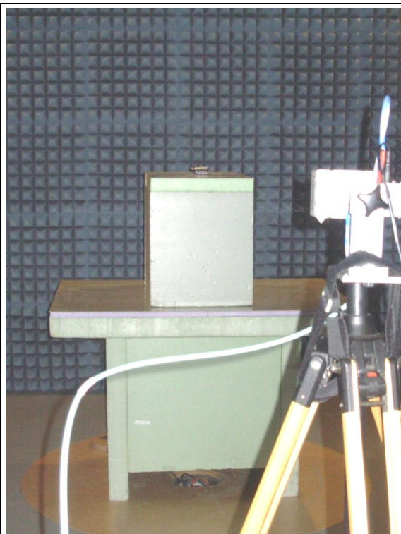
Figure 10: Measurement set-up for radiated measurement > 1 GHz acc. following sections of the report 1112-11-EE-11-PB001: 4.5.3; 4.5.4 and 4.6.2
