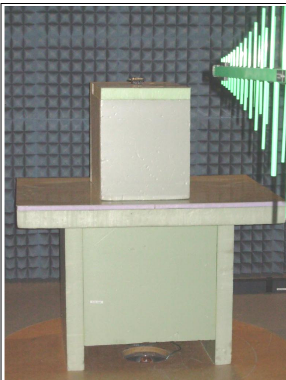
Figure 9: Measurement set-up for radiated measurement > 30 MHz and < 1 GHz acc. following sections of the report 1112-11-EE-11-PB001: 4.5.2 and 4.6.1
