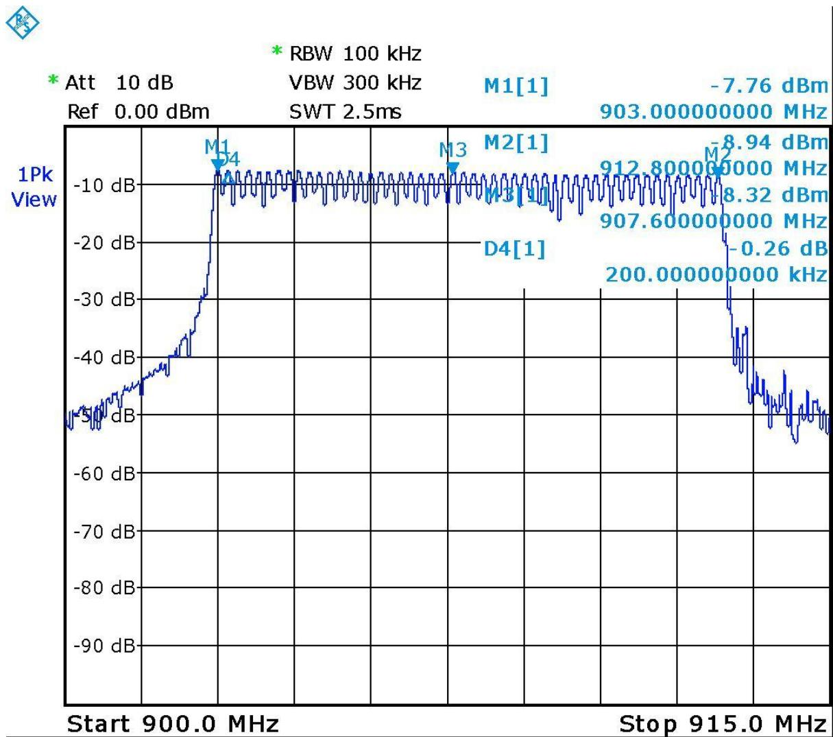
50 hopping channels between 903 MHz and 912.8 MHz with a channel spacing of 200 kHz
