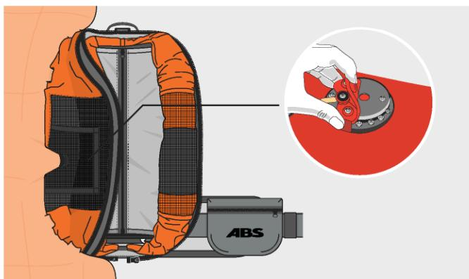
After an activation you find the Venturi nozzle to deflate air behind the orange mesh Net on the airbag. Push the red release flaps on the backside of the venturi nozzles and compress the airbags at the same time until they are completely empty.
