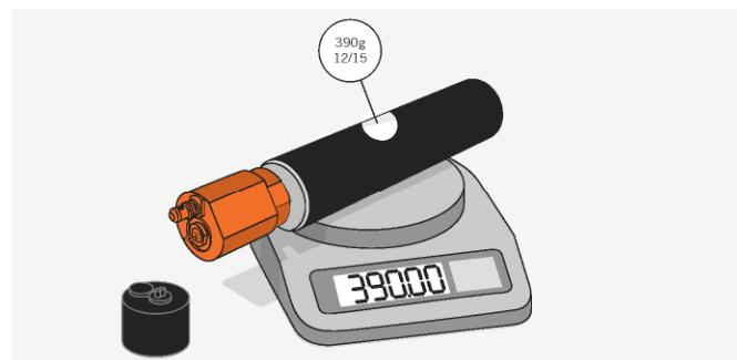
Check the inflator regularly by weighing it without the protective cap. The weight details are specified on the bottle. Tolerance limit +/- 5 grams.
