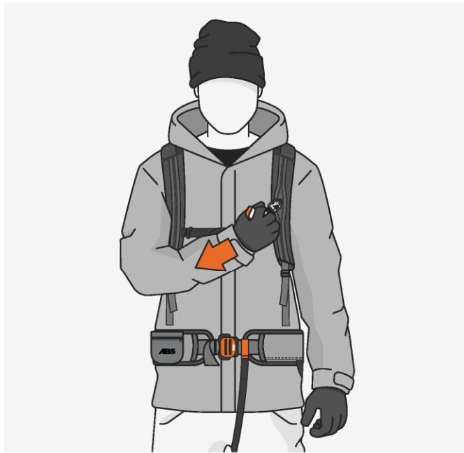
The required activation force is approx. 6 kg (60 N). The airbags will not inflate; only the tensile force is simulated. If test activation was successful, the top LED lights up white for 3 seconds and then returns to flashing red.
