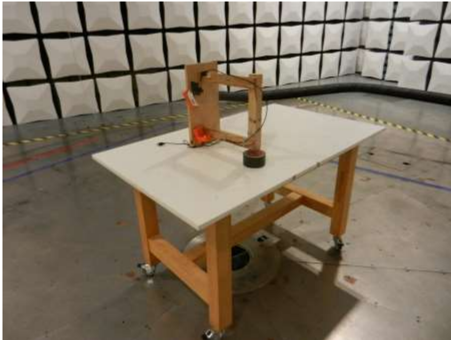
Figure 10: 30 MHz – 1 GHz: EUT on long side
