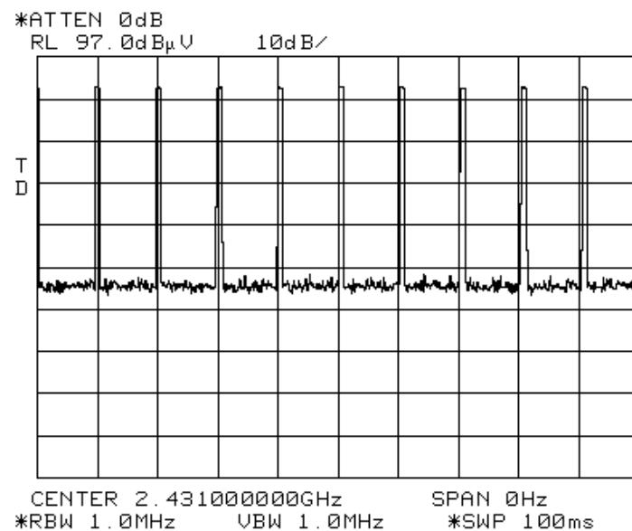
Duty Cycle correction =  $20 \log (T_{on}/100 \text{ mS})$
