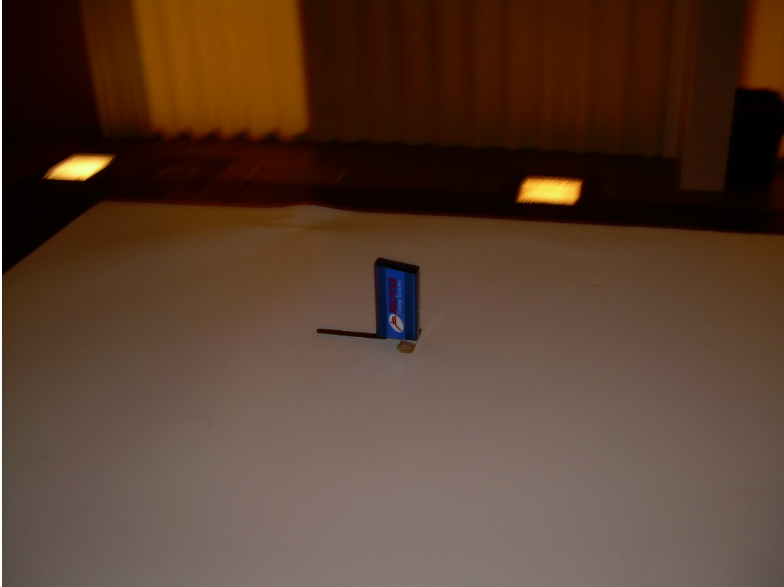
Photograph 3 - View of the Radiated Emission Test Setup (On-Edge Alignment)
