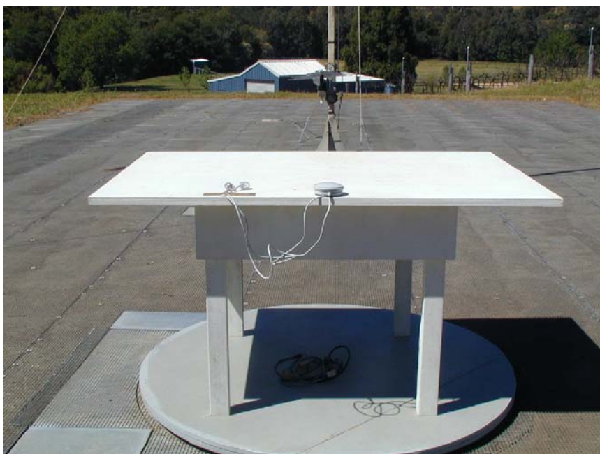
Radiated Emissions Test Setup (EUT Rear View)
