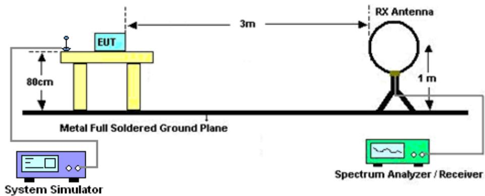
For radiated test from 30MHz to 1GHz
