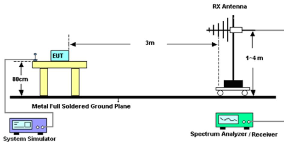
**For radiated test above 1GHz**
