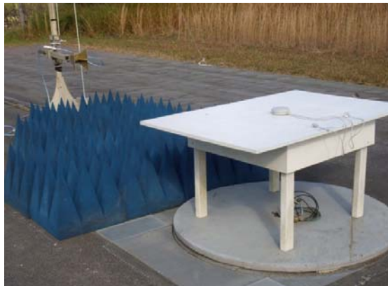
Radiated Disturbances 1000MHz – 4500MHz (3 metres)
