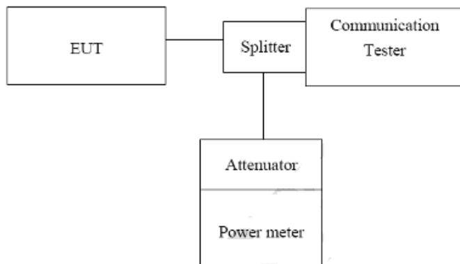
Measurement Setup for testing on Antenna connector.
