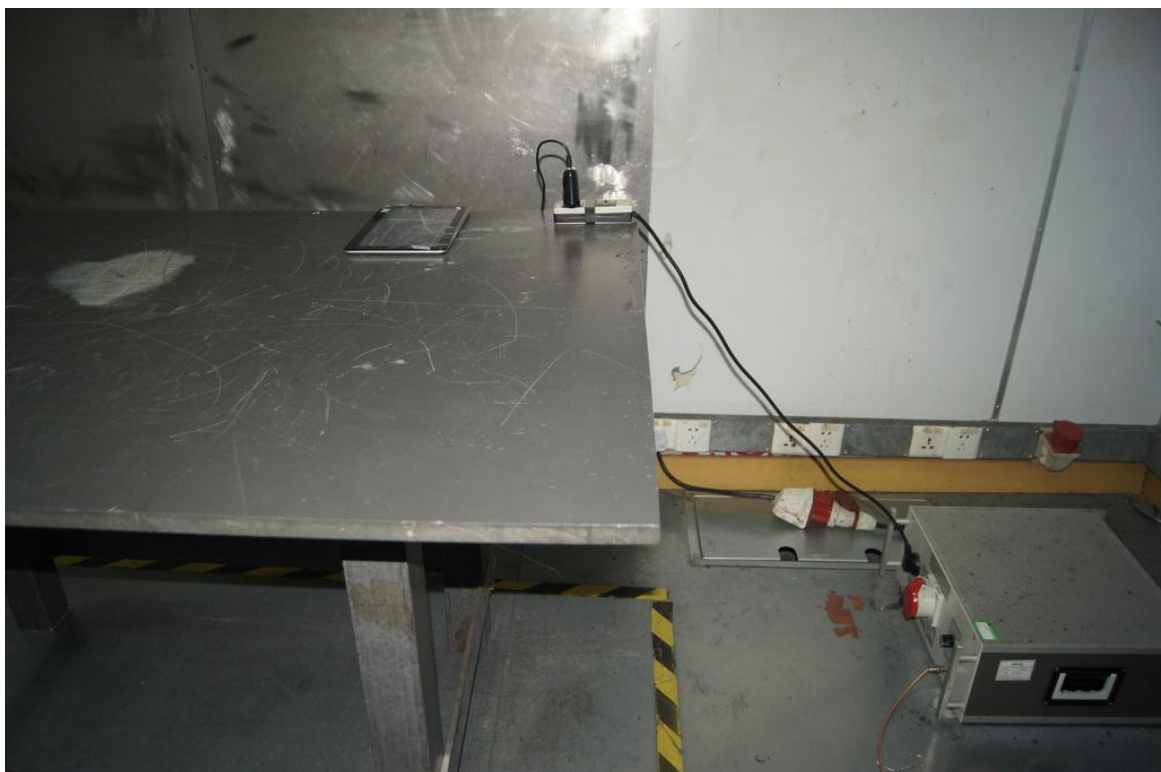
Photograph 4: Setup for Conducted disturbance
