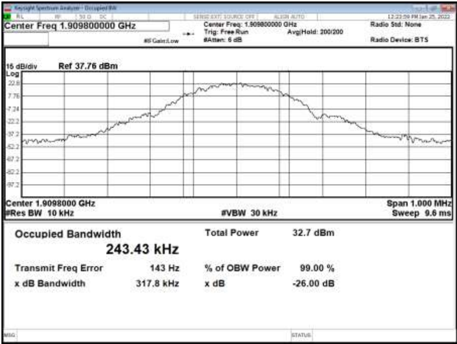
Figure 43 - 26 dB Bandwidth, 1909.8 MHz
