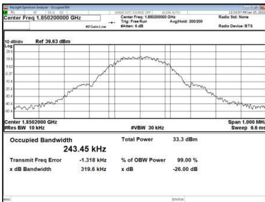
Figure 41 - 26 dB Bandwidth, 1850.2 MHz
