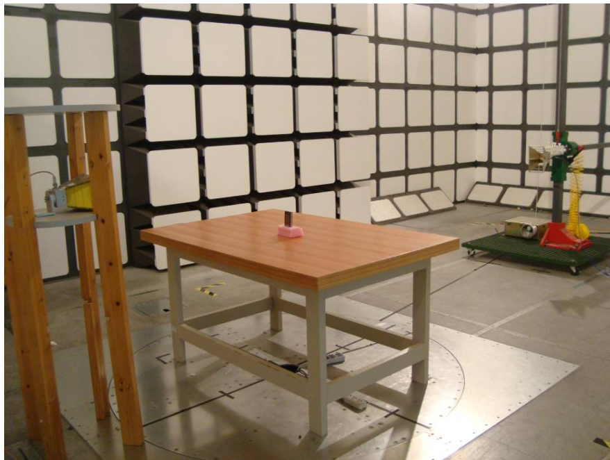
Above 1 GHz: Spurious Radiated Emissions - Rear View
