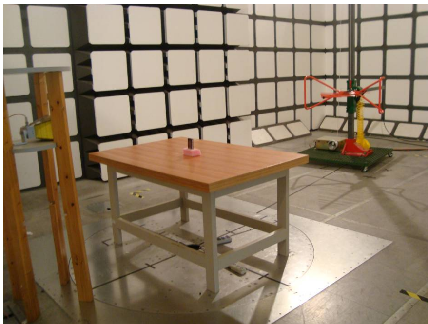
Below 1 GHz: Spurious Radiated Emissions - Rear View
