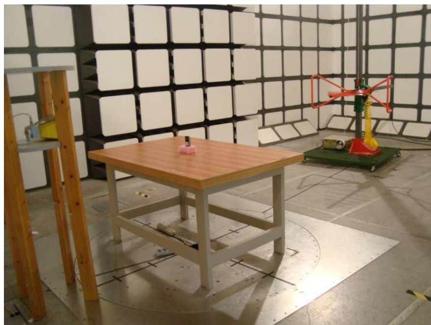
Below 1 GHz: Spurious Radiated Emissions - Rear View
