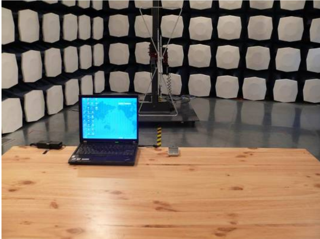
Picture 2 Radiated Emission Test setup
