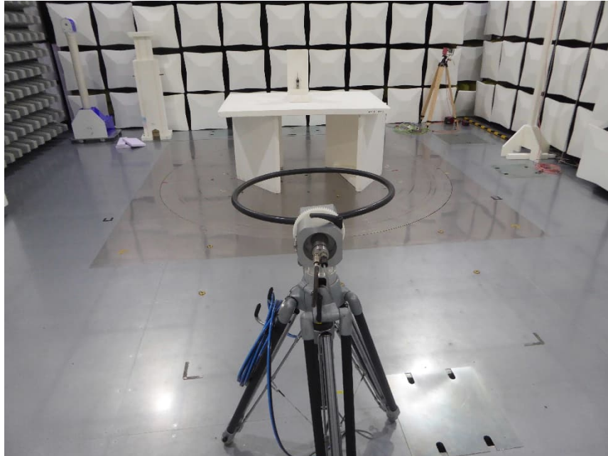
Antenna Position 3 – grund-parallel Test setup semi-anechoic chamber M276 Preliminary measurement
