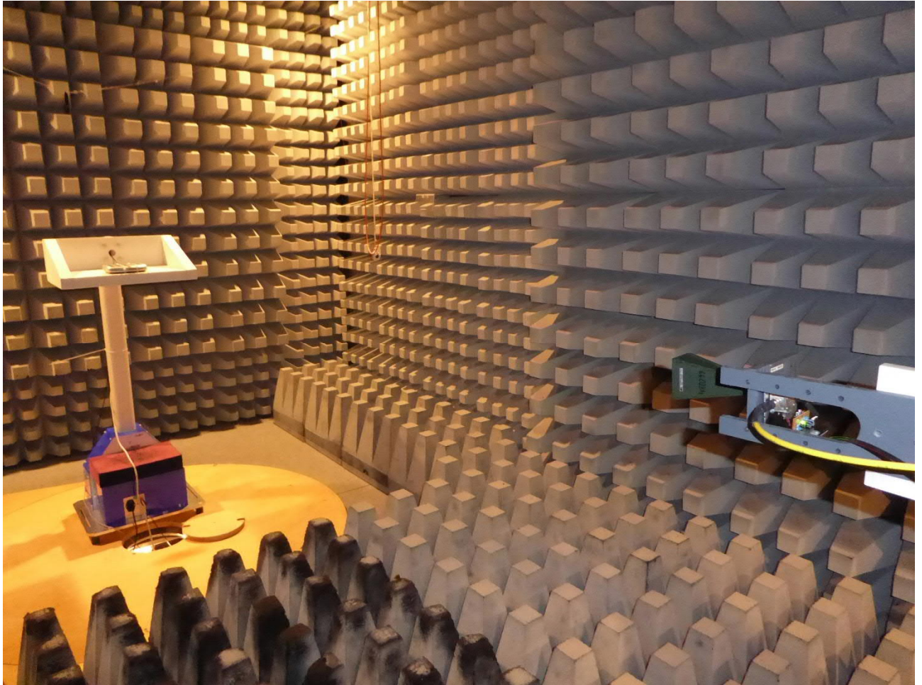
Test setup fully anechoic chamber TX spurious emissions from 18 GHz – 26.5 GHz
