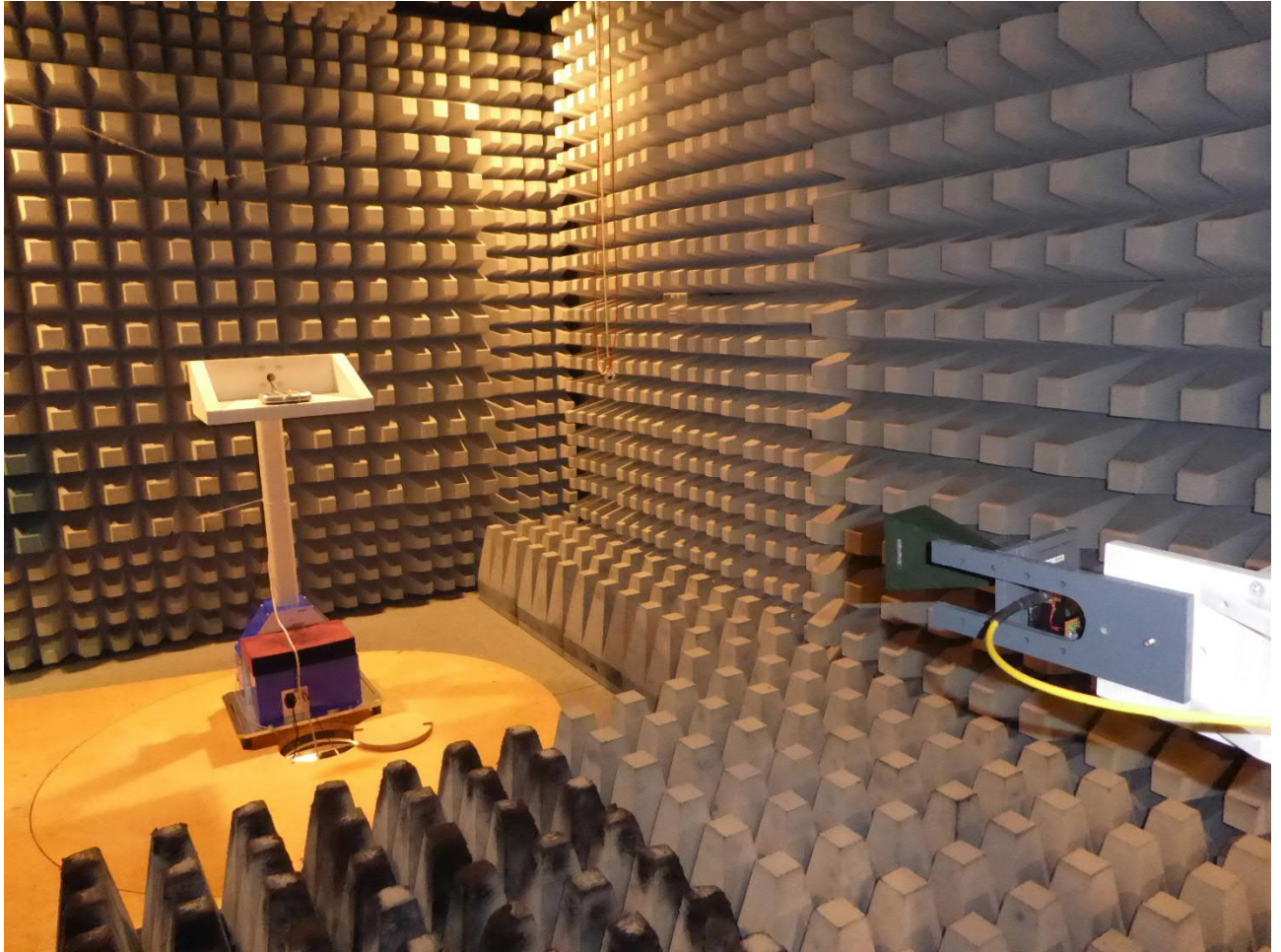
Test setup fully anechoic chamber TX spurious emissions from 12 GHz – 18GHz
