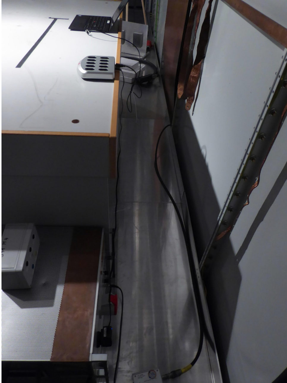
Test setup AC power line conducted
